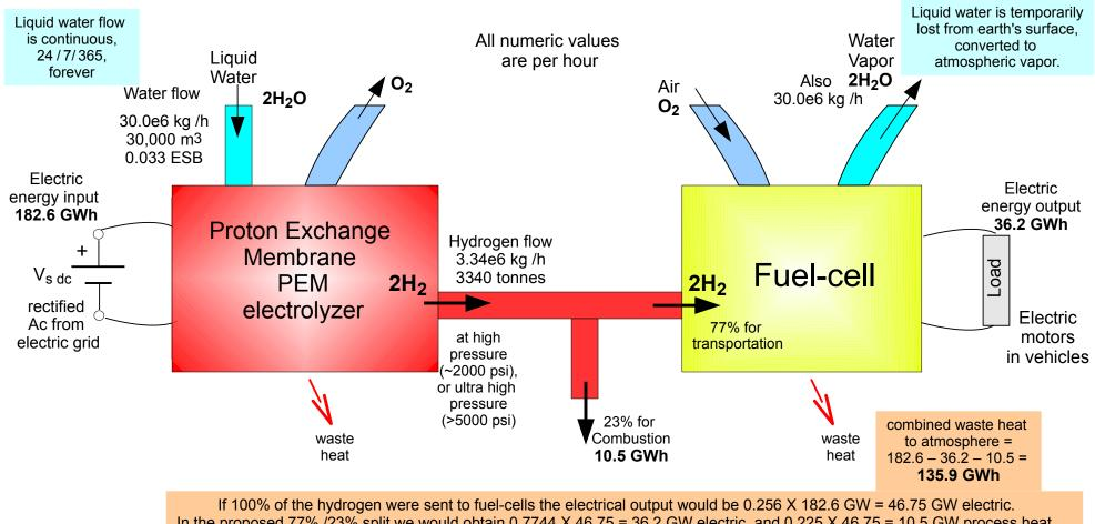
In the proposed 77% /23% split we would obtain 0.7744 X 46.75 = 36.2 GW electric, and 0.225 X 46.75 = 10.5 GW process heat. If all the process heat could be utilized for industrial product with none lost to the surroundings, the overall waste heat of the Plan's entire hydrogen system would be 182.6 – 46.75 = 135.9 GW. Of that, 0.7744 X 135.9 GW = 105.2 GW is caused by the trucks' fuel-cell propulsion.
